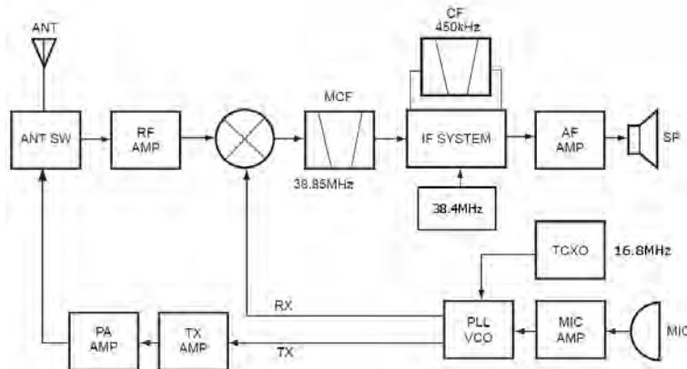
Fig. 1 Frequency configuration
